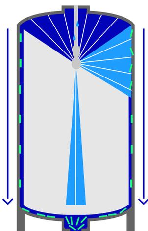
GEA's slow rotating cleaners use targeted flat or round jets to project the cleaning solution onto the vessel walls. These units operate at higher liquid pressures than traditional free rotating units but, because of their design, maintain slower rotation speeds. This enables these devices to impact greater cleaning forces onto the vessel walls than the free rotating units. As the rotation is slowed down, the spray jets have an increased dwell time, providing even more cleaning power.
