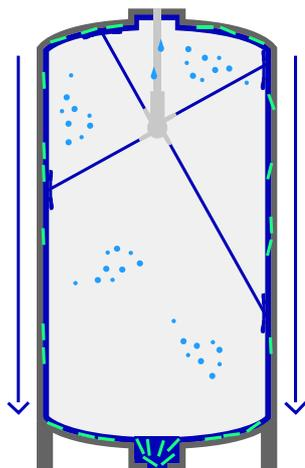
Orbital cleaners from GEA create spray patterns that optimize the cleaning performance on the vessel walls.
