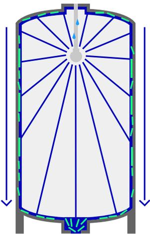
The cleaning of vessels within soiling classification I requires a liquid distribution which delivers large volumes of fluid simultaneously over the complete vessel. Static spray balls apply lower mechanical force so they rely on the liquid running down the vessel walls to create surface friction or to dissolve the residues.
