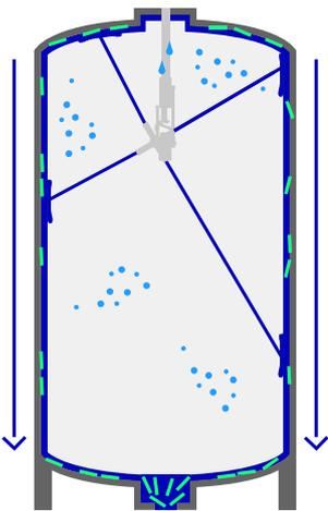
GEA's unique range of index cleaners provide highly effective cleaning performance through their piston-operated index mechanism. The advantage of this type of cleaner is that large amounts of energy can be applied by the slow moving operation, directly onto the vessel walls.
