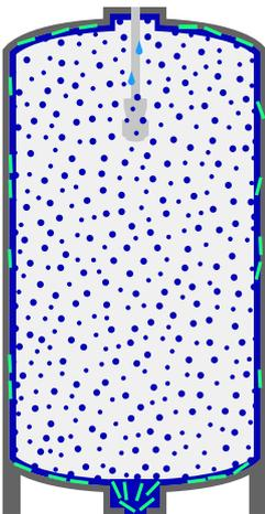
All our free rotating cleaners are driven by the wash liquid entering the cleaner through the inlet. Using contoured internal flow paths allows to minimize the internal pressure- and energy drops while directing the liquid into high velocity droplets. This is done via a series of specially shaped rotors that effectively distribute the liquid in the designated spray patterns.
