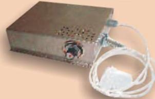
Detail of thick film heating element with control
