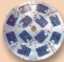
Heating of bottom by heating elements and walls by band heaters
