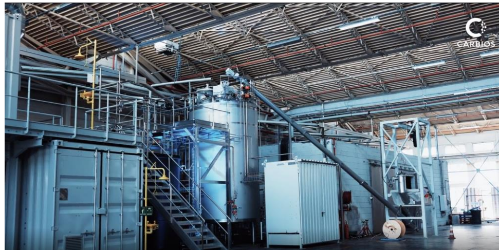
Carbios depolymerization Unit for the conversion of PET waste into monomers
