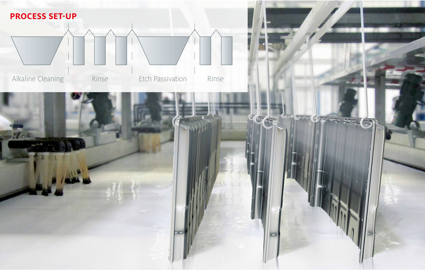
Aluminum battery pack top covers immersed in a treatment bath
