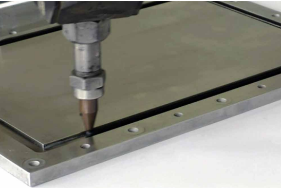
Butyl gasket (LOCTITE ESB 5100)
