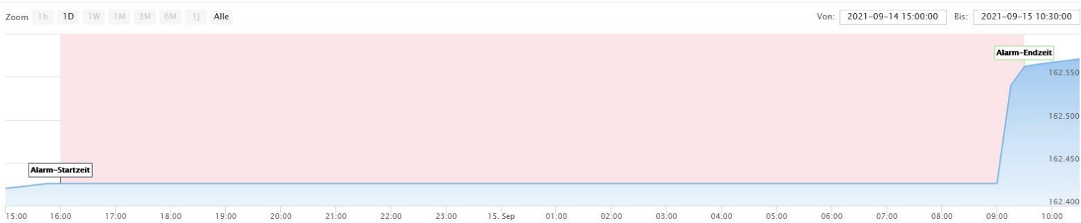
Example of an alarm triggered by the sensor failure detection surveillance
