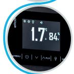
Digital control of temperature, humidity and ventilation (controller DIXELL XH360L)
