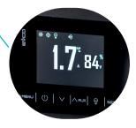
These changes are also visible on the display of the cabinet, which shows the real values of temperature and humidity at a given moment and not fixed set points.
