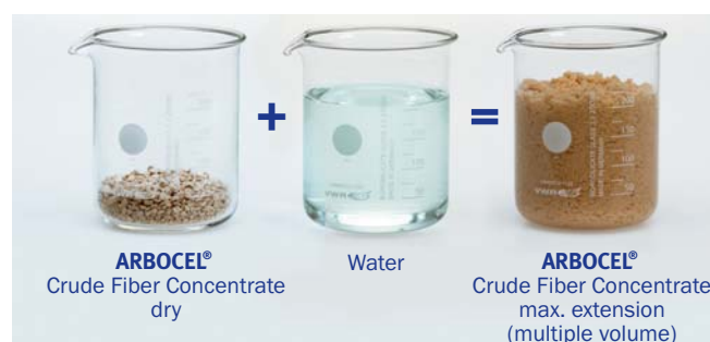
Fig. 11 Test for swelling capacity of HPC-fibrillated Lignocellulose in water (JRS, 2012)
