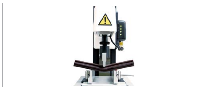
Pic. 3: Measurement of Mechanical Resistance in a Dental Chew - Three Point Bend Test (Stable Micro Systems)
