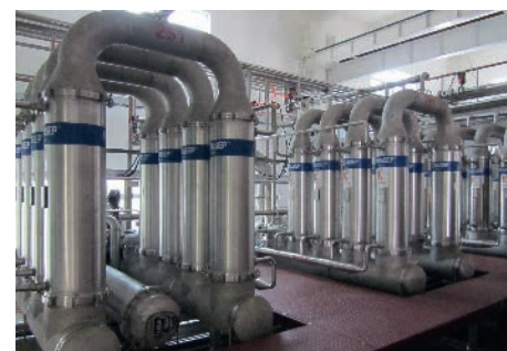
Filtration unit for antibiotics production
