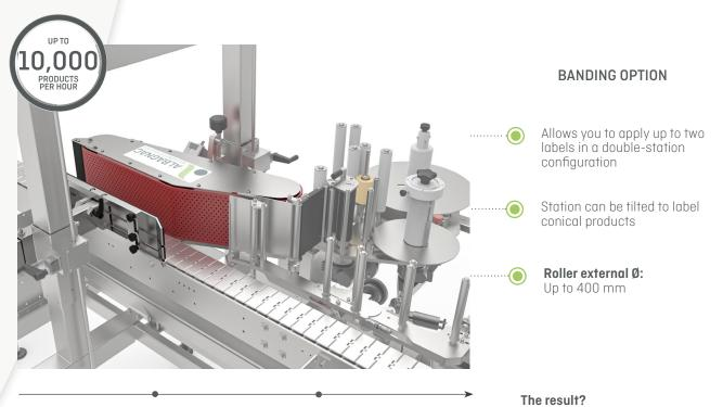
Label drop vial aspiration over a perforated belt Smoothing by non-stop rotation of the product against a belt The result:
