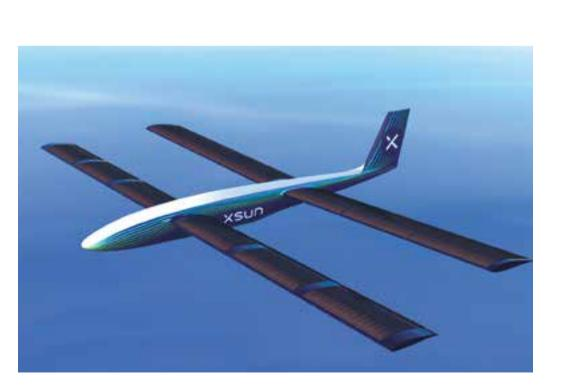
XSUN French company XSun has designed, tested and demonstrated the capabilities of its long-range, solar-powered drones.
