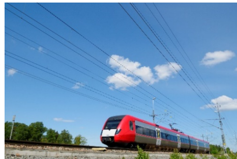
An overhead electrified train. Many countries in the EU have extensive electric public transit networks.
