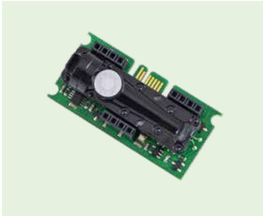
**EE894****CO<sub>2</sub> Module Measures Four Climate Parameters**
