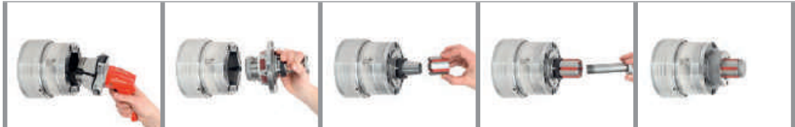
Remove clamping head Insert MANDO Adapt T211 Fit on segmented clamping bushing Screw in draw bolt Clamping device set-up
