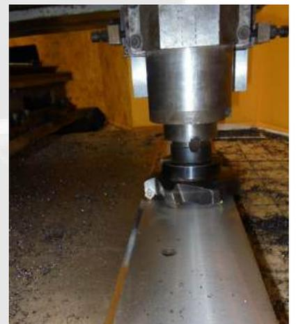
Fraisage de plaque TKJ / TKJ Plate Milling
