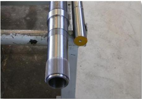
VIS CREUSE AVEC CANNELURES
