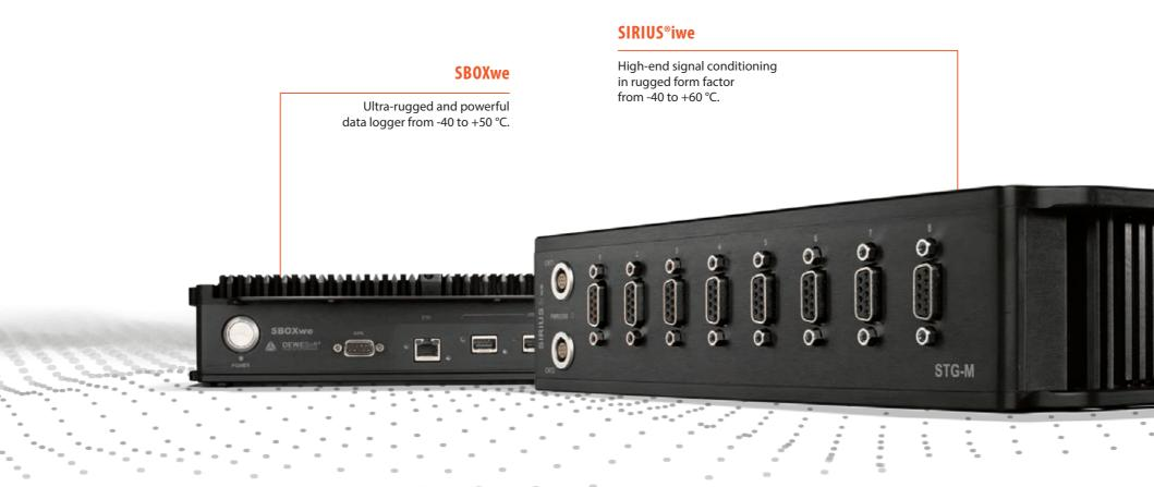
Extremely rugged (IP67 degree of protection) and fully isolated data acquisition system for the most demanding testing in harsh environments. High-precision, high-dynamic, and high-bandwidth for all types of analog signals from IEPE to strain gages.
