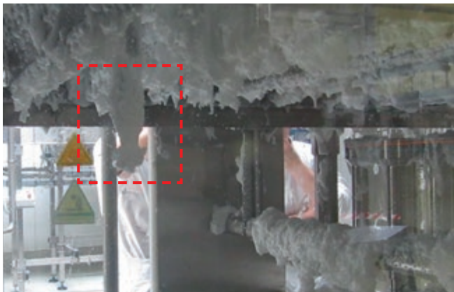
Figure 7: Foam cleaning with a Lechler PVDF MicroWhirly
