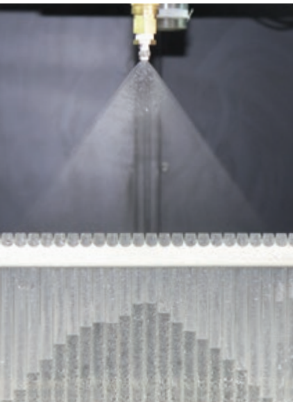
Figure 13: Liquid distribution measurement
