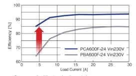
Compared with standard model Efficiency increased by approx. 8% In the light load range
