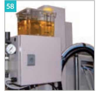
000947 Minimal lubrication system 1.3 liters
