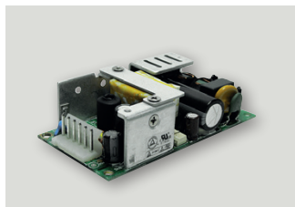
Medline 60 OBJ07 Series 37.5-64W Open frame 2" x 4" Universal input 90-264VAC Multiple output 5, 12, 15, 24 or 48VDC
