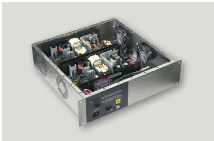
400W AC/DC open frame quad output power supply for diagnostic system.
