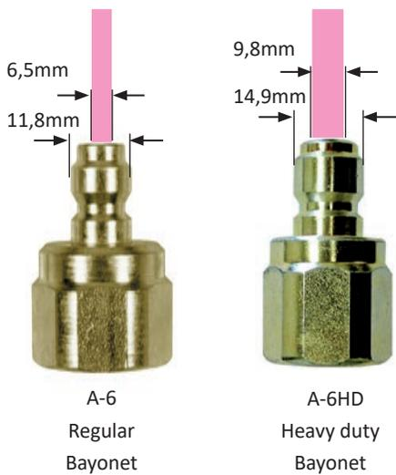
Specially for the large wire diameters used in Submerged Arc Welding Wire Wizard developed a range of connectors with a large Bayonet. These HD connectors provide a larger feedthrough than the regular connectors and avoid the connector passage becomes a bottleneck in your system.
