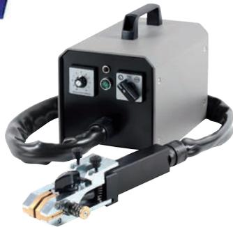
Avoid losing lots of time with feeding in a new wire. Due to the large wire diameters used in the submerged arc business feeding in a new wire can be a very time consuming job. All this time your production is down. With this small, hand-held butt welder the wire-ends can be welded together very easily. Once the welding is done the feeder motor will do the rest and welding restarts much quicker as before.
