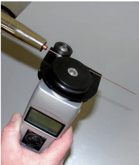
HHSS-12 obtaining measurement at the torch end
