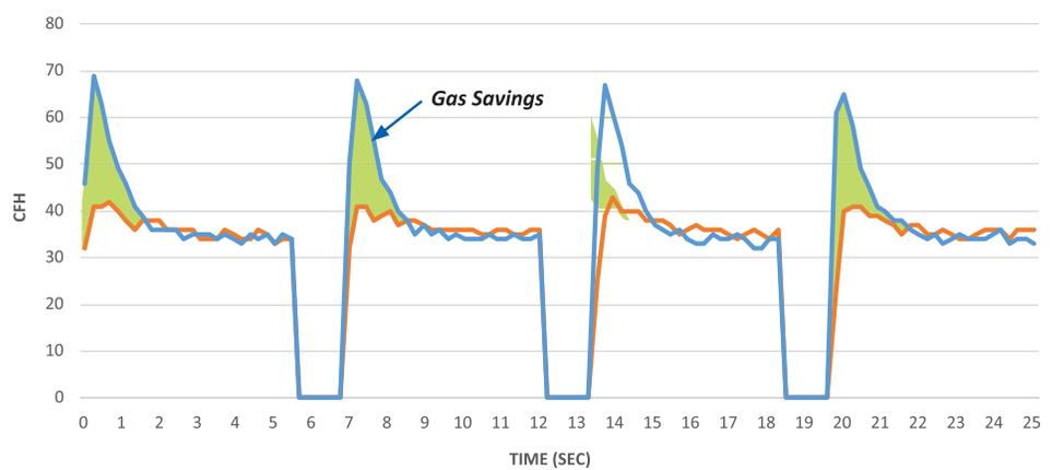
Gas savers available for the inlet or outlet side of gas solenoid
