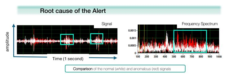
The raw signal comparison allows to identify the **temporal and frequential signature** of the anomaly. By analysing the **physical phenomenon** linked to suspect machine behaviour, our system can guide **appropriate corrective actions**.
