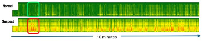
A second detailed color-coded representation (1s resolution) enables precise **event comparison** and a **real-time tracking** of the machine health.
