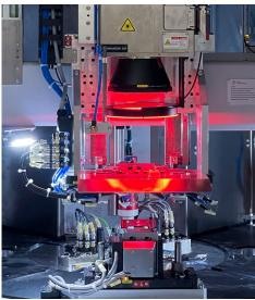
More and more power tools and gardening equipment are being built with compact and lightweight battery systems thanks to new battery technologies. Without cables to the power socket, they can thus be used on the move and enable efficient, ergonomic work. In manufacturing, laser welding is used in the assembly of battery modules, especially for cell contacting. The contacting of battery cells by laser is characterized by high reliability and low costs per cell.
