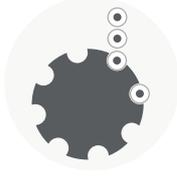
Bottles immobilised by an 8-branch star during transfer between the various machine stations
