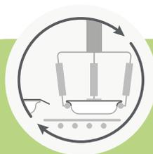
Synchronous dynamic smoothing: Smoothing and folding down the label onto the product with mobile, synchronised equipment at the same speed as the
