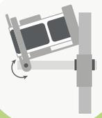
Optimised adaptation to your conveyor belt thanks to a base that can be adjusted in height and transversally
