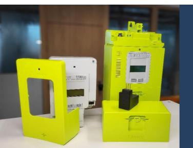
The TeeKY® seamlessly retrieves TIC data from Linky smart meters, whether single-phase or three-phase models.
