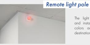
The light pole is connected to the robot (via a specific box) and installed in your establishment. It makes it possible to display colors according to the state of the mobile robot (arrival at destination, in error, etc.) in order to visually warn users.
