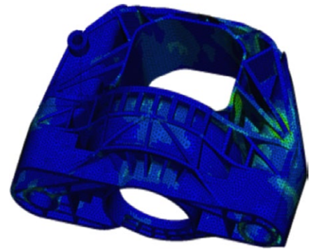
40% mass saved by metal replacement on engine mount
