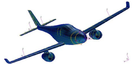
Multiple rotors with external superelements
