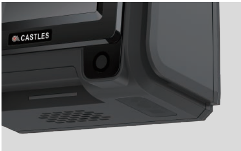
Camera and optional barcode scanner for data capture
