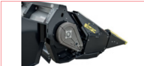
Oil-bathed cylindrical gears auger transmission
