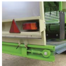
Conveyor belt with control tension device
