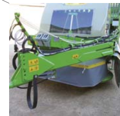
Double drawbar reinforced frame
