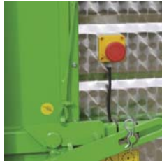
Automatic release emergency button on both sides
