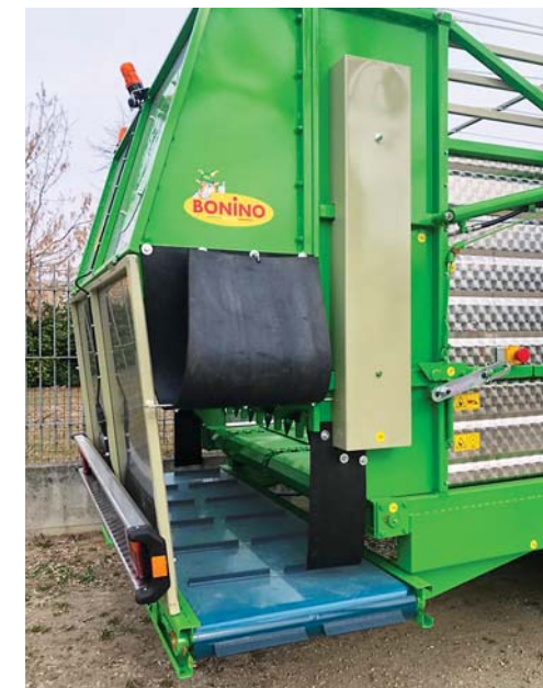
LATERAL UNLOADING BY PROPER DOSING WITH RUBBER BELT L=750 mm MANUALLY RETRACTABLE
