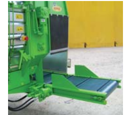
Conveyor belt extension
