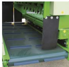
Conveyor belt width: 750 mm Side conveyor belt
