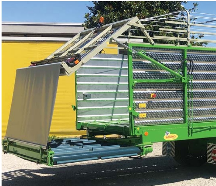
LATERAL UNLOADING CONVEYOR L=1 400 mm HYDRAULICALLY RETRACTABLE
