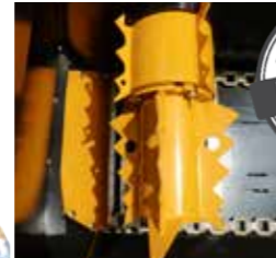
Agitating roller with hydraulic opening door: regular and fast feeding.
