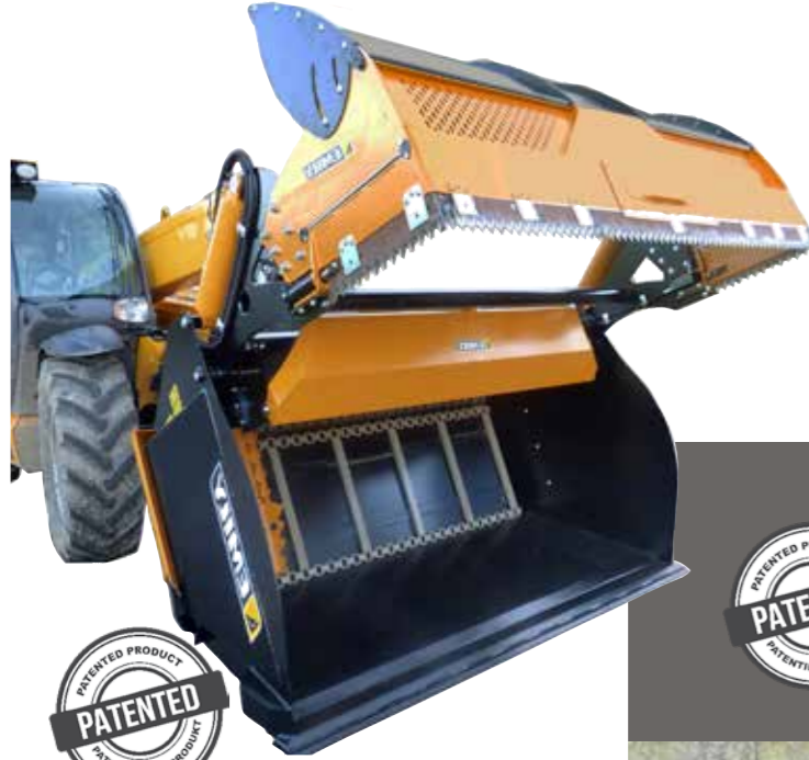
Agitating roller with hydraulic opening door: regular and fast feeding.
