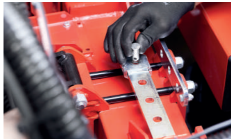
Quick adjustment of the row distance by rods with locking pins.
