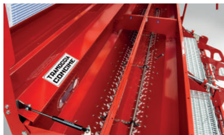
ARIZONA KOMBI is equipped with a big tank divided into two for seed and for fertilizer.
