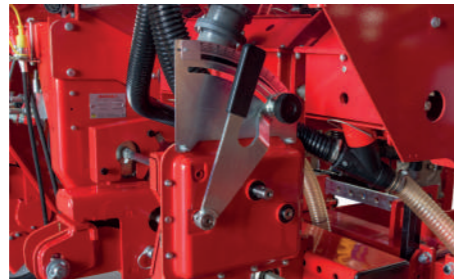
Centralized fertilizer quantity adjustment with continuous gearbox in oil bath.
