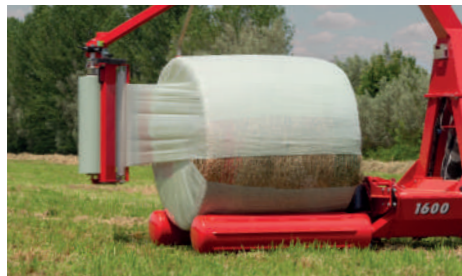
Satellite arm for a fast and uniform wrapping.
