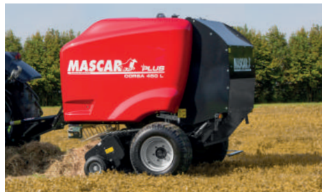
The hydraulic pick-up is available in sizes 170 cm and 200 cm.
