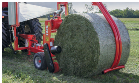
Hydraulic loading central fork in the 2100S version.
