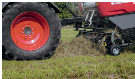
Rotary feeder available with or without 15 or 25 knives CUT system.
