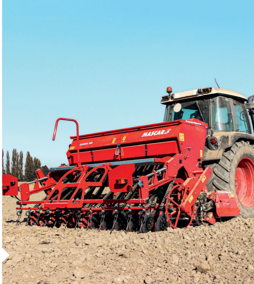
FLORIDA COMBI is equipped as standard with the packer roller - power harrow.
