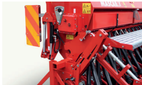
Centralized coulters adjustment.
