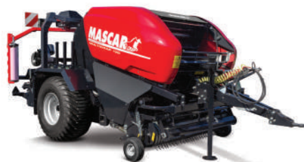
Fast wrapping system with double satellite arm.
