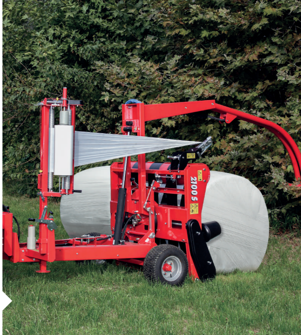
Hydraulic loading central fork in the 2100S version.
