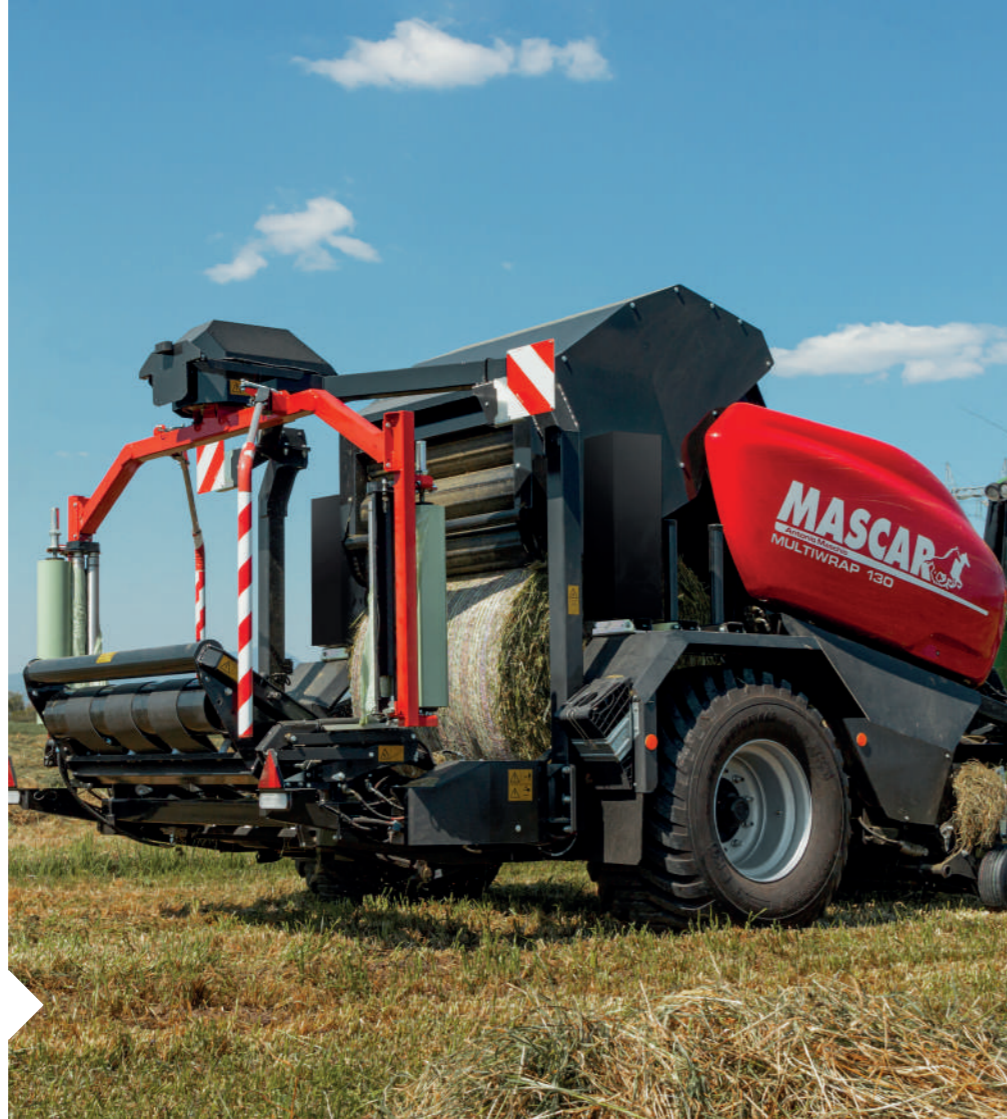
Rotary feeder available with or without 15 or 25 knives CUT system.
