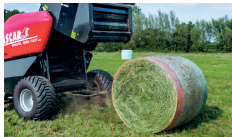
Compression chamber with 18 rollers.
