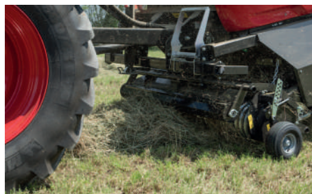
Rotary feeder available with or without 15 or 25 knives CUT system.
