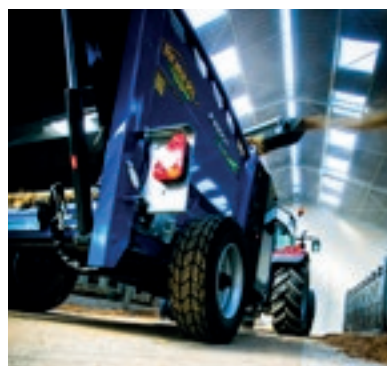
P700 GT Type de goulotte: Tournante 300° Type of chute: Turning 300° Type stortgoot: Draaiend over 300°
