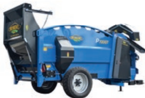
P700 GT Type de goulotte: Tournante 300° Type of chute: Turning 300° Type stortgoot: Draaiend over 300°
