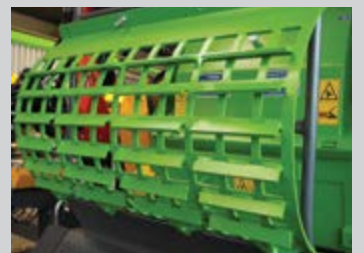
Grilles de calibrage : 25/25mm, 35/40mm, 45/60mm, 60/80mm
