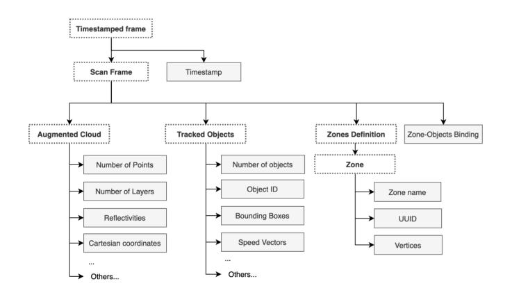
The Augmented LiDAR Box<sup>©</sup> delivers its output using OSEF, a serialization binary format, based on <u>TLV-encoding</u>.
