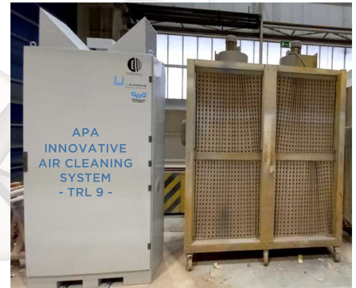
OLD SYSTEMS WITH PAPER FILTERS (still in use)
