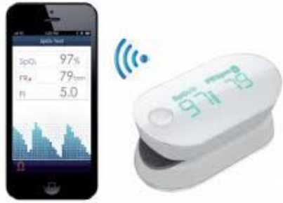
Connected Oxymeter Remote monitoring of oxygen saturation (SpO2) by pulse oximetry
